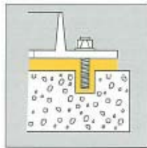
Machine Base Grouting
